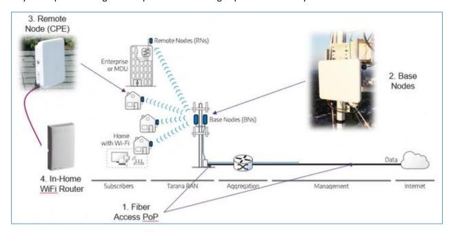
Each Township will have an Internet Peering connection connected to the Fixed Wireless Access Point/Broadcast Tower site, as depicted in the Fixed Wireless Access Architecture diagram below. The PTP connection may or may not be used depending on the location of the Internet Peering Point in relations to the broadcast tower. One location includes a PTP to extend the network from the Internet
